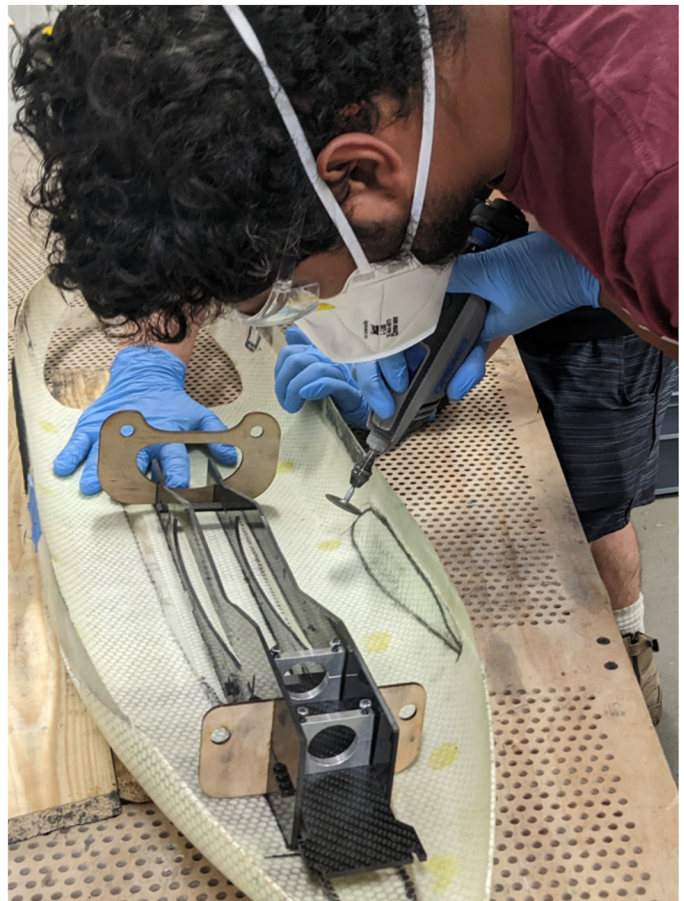
Cutting the wing slots on V2 (Phoenix)
